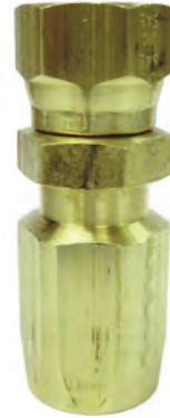
500B-10 #10 JIC X 15/16" OD hose end fitting, reusable, for use on 1/2" ID rubber hose
