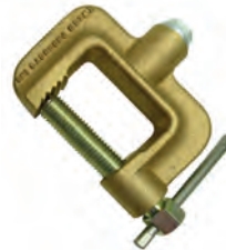
Ground clamp GC-600-50 600 amp, c-type 98% copper alloy, 2.5" opening
